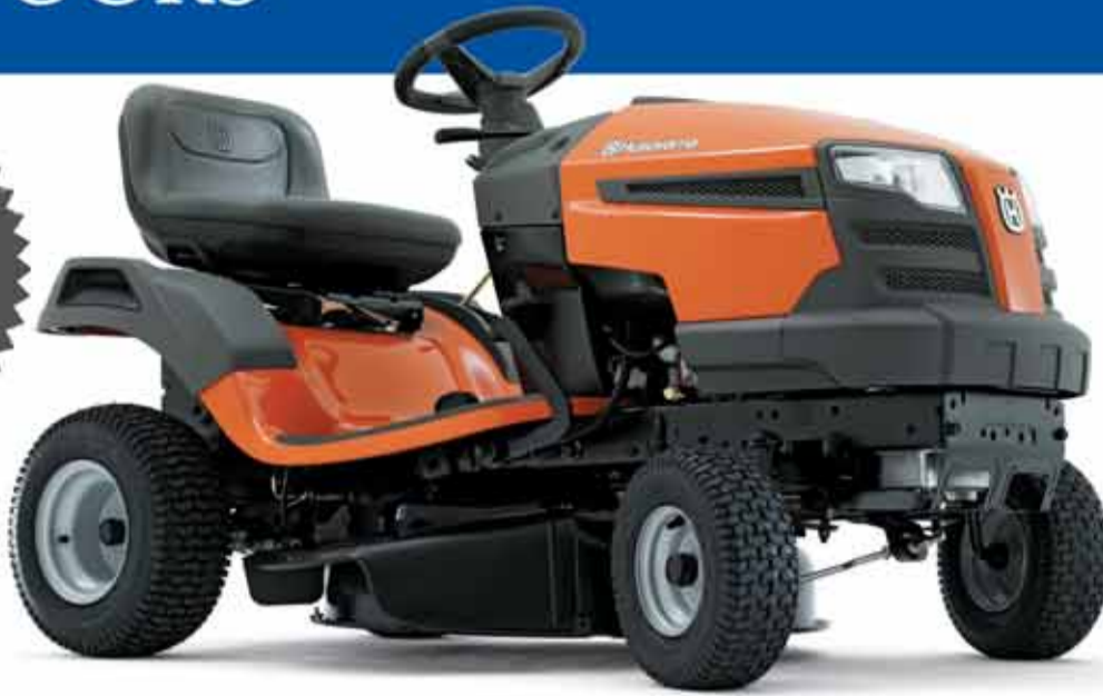
LTH126 Tractor Briggs & Stratton - 12.5hp - Foot-pedal Hydrostatic - Side-discharge 77cm (30") cutting deck.
