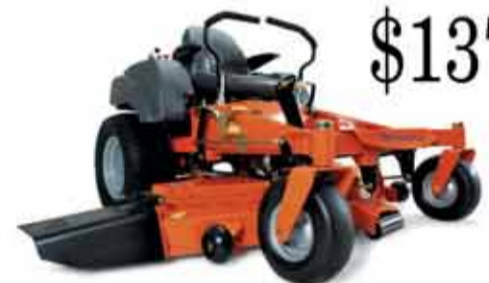
MZ25 Zero Turn Kohler Courage Pro 25hp - Choice of 52" or 61" fabricated 10 gauge cutting decks. Price includes 52" deck
